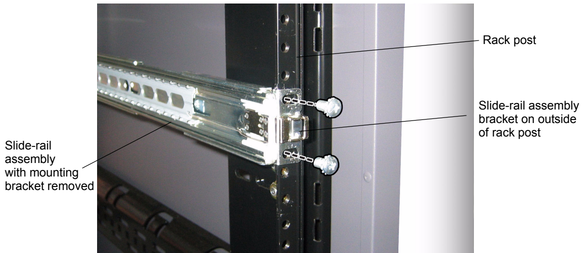
FIGURE 1-3 Slide-Rail Assembly Mounting to Rack Post
